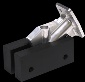
Mors doux MarkForged: 40€ - Usinage: 250€
